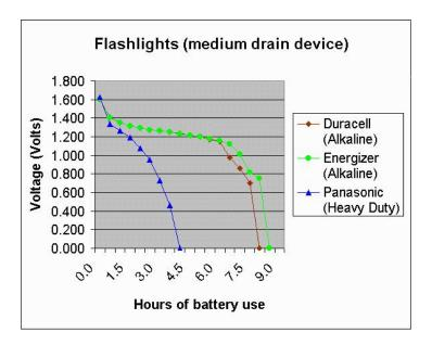
Fig. 1. Graph of voltage vs. hours of battery use in flashlights for three brands of batteries.
